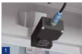
Safety guard monitoring
